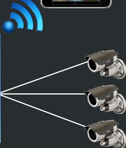
Up to three additional cameras can be added including RS485 telemetry (if required). Ideal for adding a further three lanes of ANPR to the one unit or a further lane plus overview.
